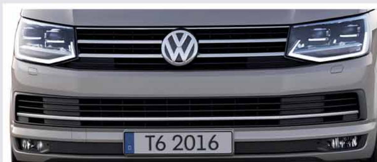
Newly designed engine cover, bumper and headlights at front
