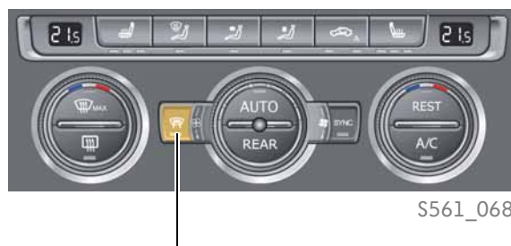
3-zone Climatronic control unit with switch for heated windscreen E180
