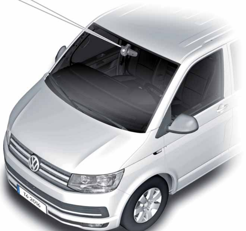
Control unit for main beam assist J844
