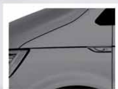
New wing panel with cut-in, rectangular turn signal repeater
