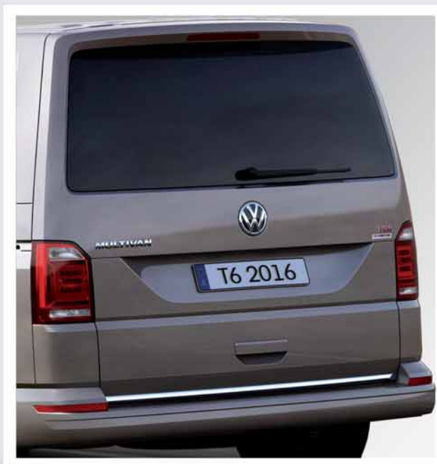
New tailgate with larger number plate panel, larger window cut-out and spoiler, New tail light clusters, optionally with LED technology and newly designed bumpers
