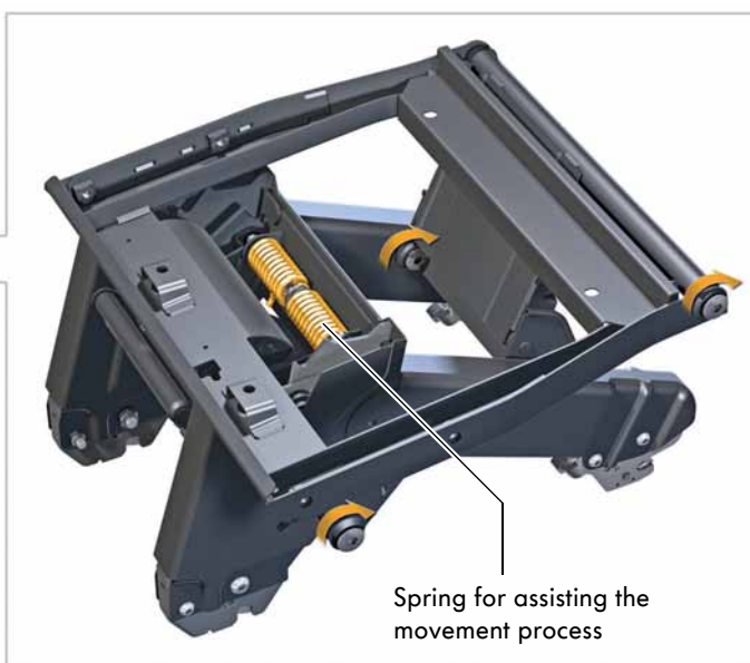
Unlocking the fold-down function of the seat frame
